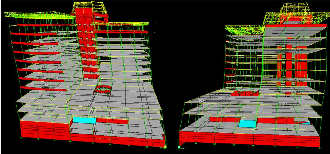
**Figure 2: Showing two views of John Wickliffe House with exaggerated deformation under east/west earthquake shaking on the left and north/south earthquake shaking on the right.**
