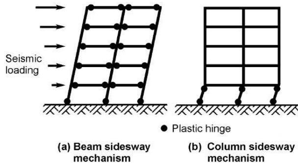
The capacity/demand ( $c/d$ ) ratio of the various members throughout the building gives an indication of which members will fail before the others under a set loading, eg the 1170.5 design earthquake loading. A capacity/demand ratio greater than 1 means the member will not fail under that loading and less than 1 means that failure will occur. Members with a lower  $c/d$  ratio will fail before those with a higher  $c/d$  ratio.
